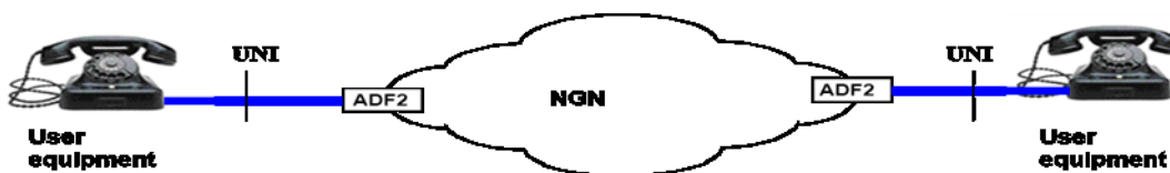
Figure 16 – Configuration of NGN Emulation
