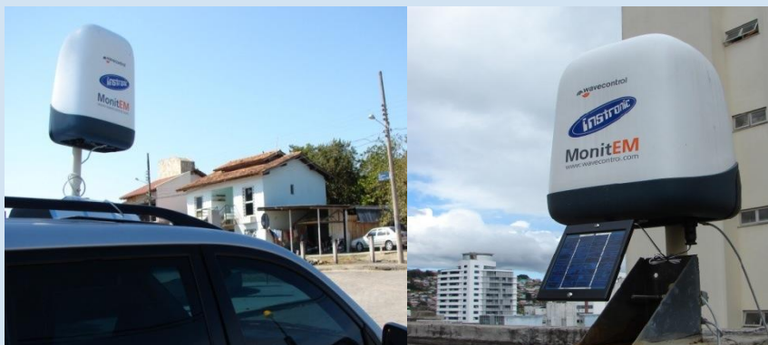
Figure 9: New EMF monitoring system assembled on a car and on a base station that uses both photovoltaic cells and a battery to guarantee continuous monitoring without an electrical power source
