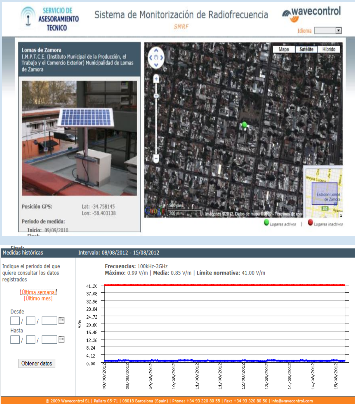
Figure 2: Example of continuous monitoring systems in Loma de Zamora based on Recommendation ITU-T K.83
