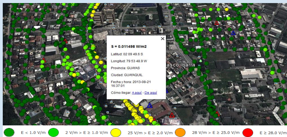
Figure 13: Example of map of the electromagnetic emissions
