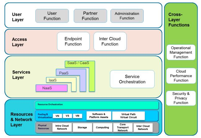
As shown in the figures, key functions of a cloud management system are divided into four layers, respectively:
