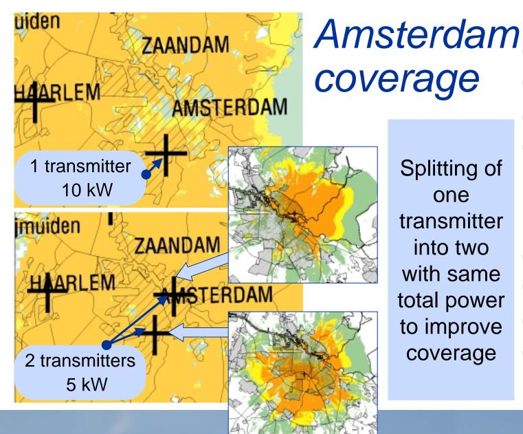
Splitting of one transmitter into two with same total power to improve coverage
