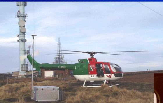
Sometimes we use a hired helicopter to check what is actually being radiated by a transmitting station
