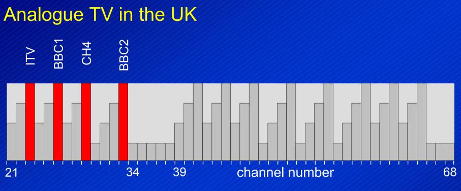
The four channels are sufficiently close in frequency to allow the use of inexpensive receiving aerials, but sufficiently separated to more easily allow the use of a common transmitting antenna
