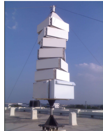
2.4 GHz LE WiMAX 24 beam Experimental Array; Bangalore, India.
