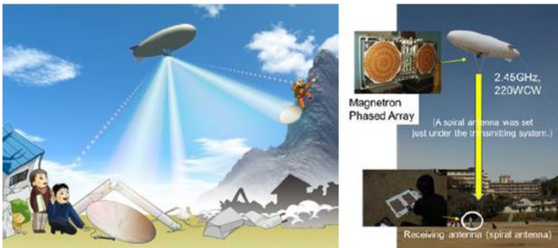
FIGURE 2.2.3 Image of an emergency UPS system and photo of experiment (2009)
