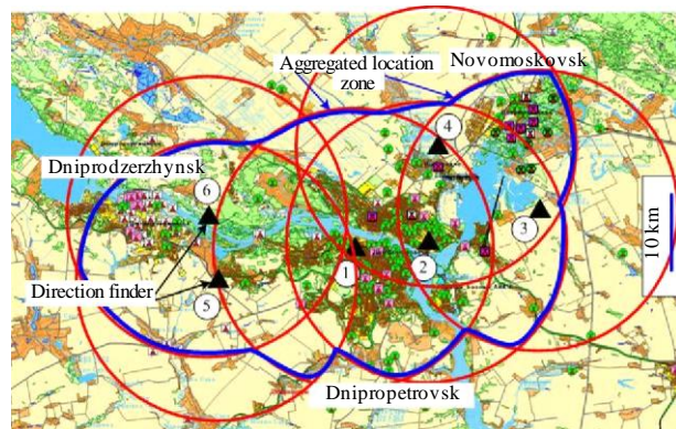
FIGURE A1-8 Aggregated location area of SMN
