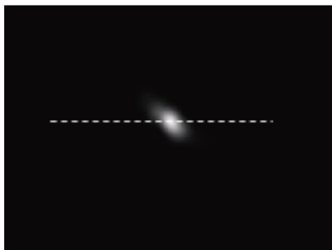
QCL beam pattern of THz array sensor with a pixel count 320x240 and a pixel pitch 23.5 \mu\text{m}
