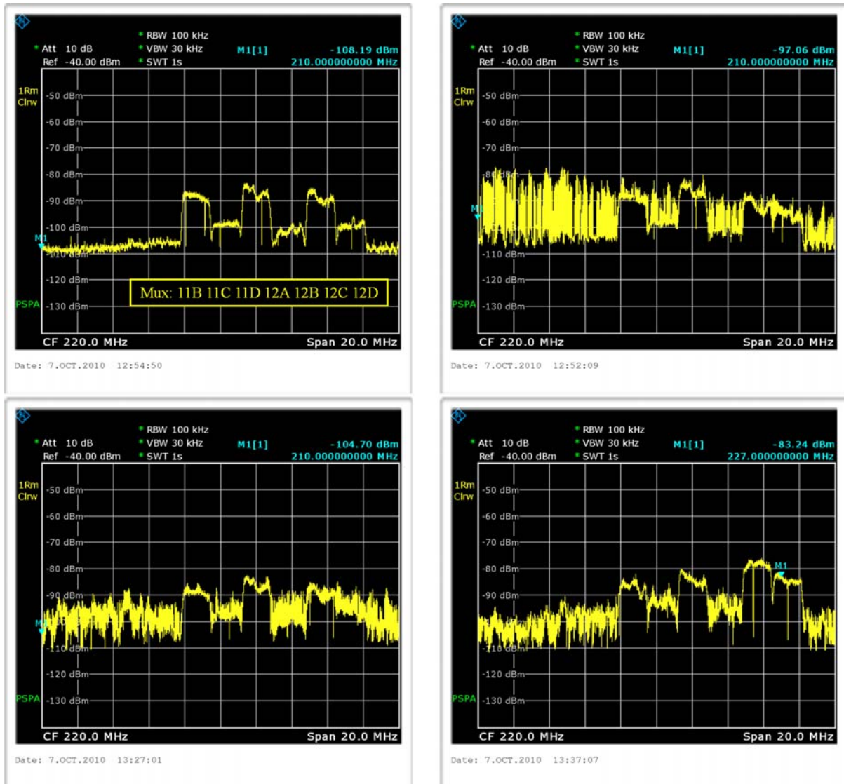
DAB multiplex spectra for different combinations of indoor receiving location and PLT network configuration
