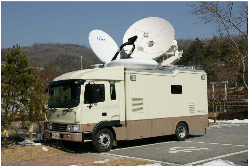
Mobile satellite radio monitoring system
