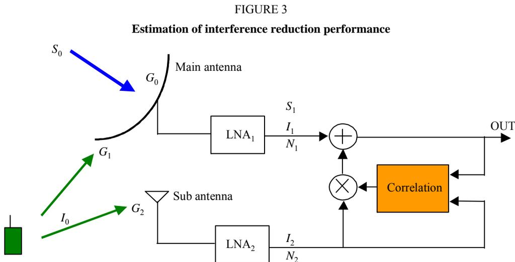
Table 1 shows an example set of parameters. Assuming that the propagation loss from the interferer to the main antenna is equivalent to that to the sub-antenna,  $I_1/I_2$  is proportional to the ratio of antenna gain between the main and sub-antenna in the direction of the interference arrival
