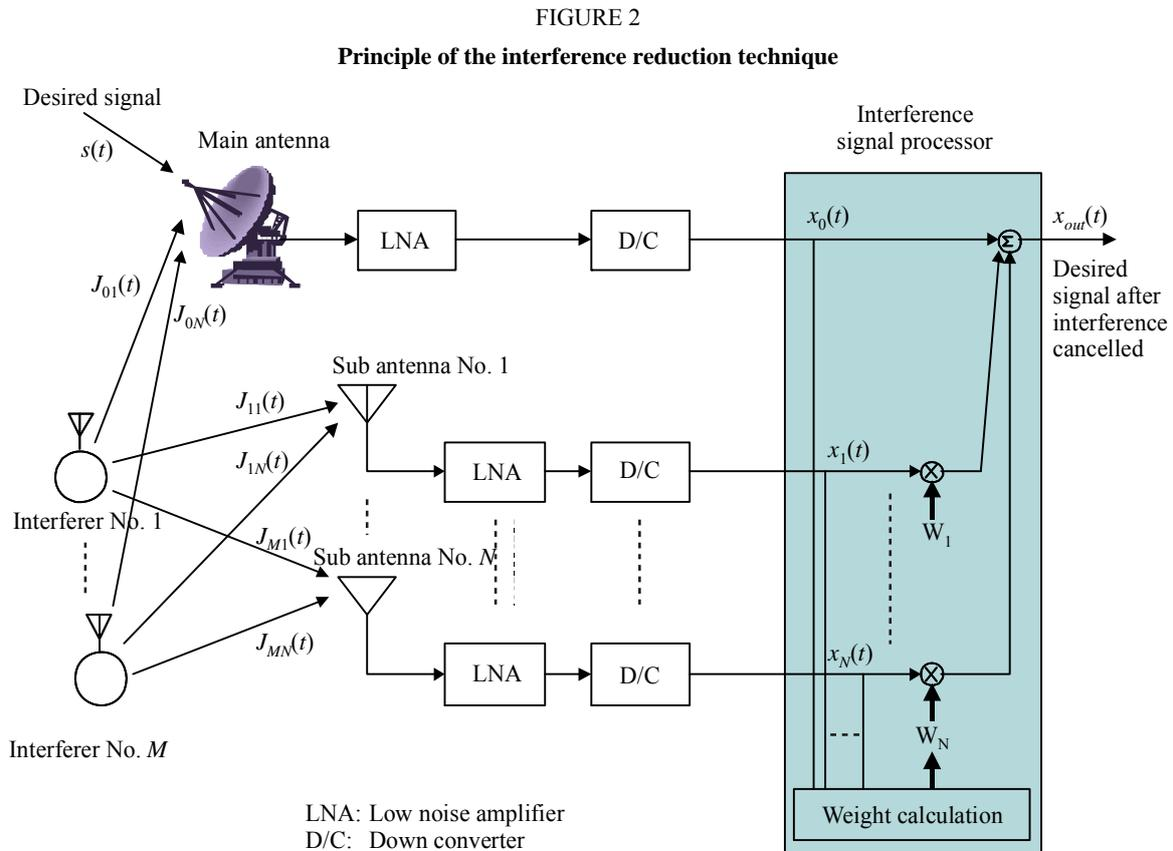
Consequently, the following signal is produced as a desired signal after interference reduction:
