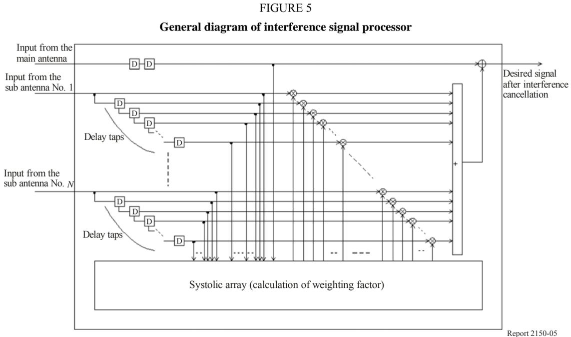
In implementing the prototype system, it is important to understand the nature of the desired and interfering signals as identified below:
