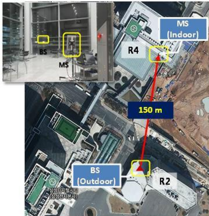
View of building penetration environments – Case 2
