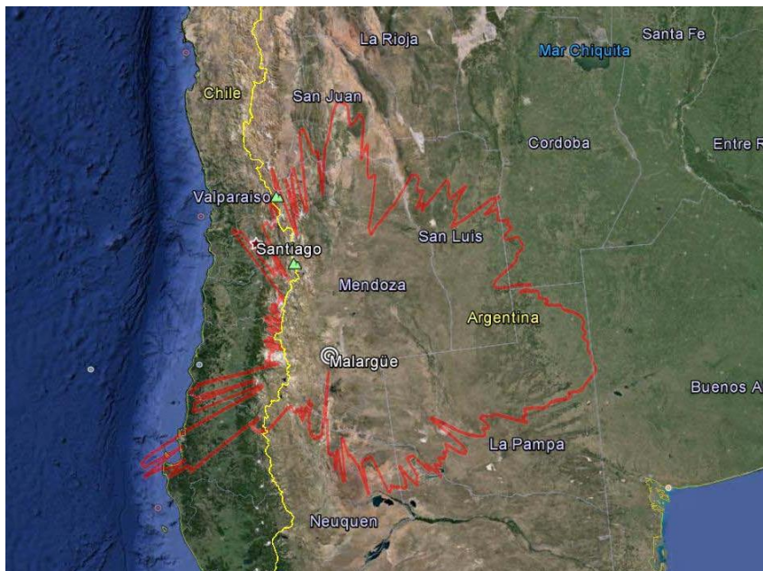
FIGURE A3-10D Map of the required separation distances between GSO MMSS and SRS earth stations at Malargüe Sur (Case 2)
