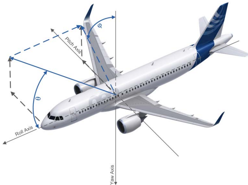
FIGURE A-3.1 Aircraft axes and angle definitions
