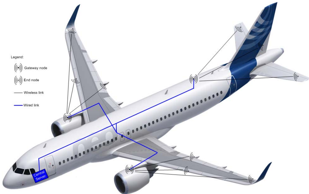
Example installation locations of WAIC transceivers outside the aircraft structure (aircraft top view)
