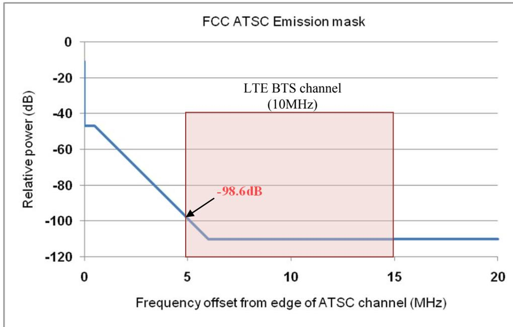
The ACS of the LTE UE to the adjacent LTE channel with the same channel bandwidth is defined as 46 dB in 3GPP TS 36.104. If it is assumed that the 5 MHz frequency offset guarantees 10 dB more than that of 3GPP specification, the ACS of the LTE BTS to the ATSC channel at 5 MHz frequency offset to the LTE channel is 56 dB. The ACIR from a ATSC transmitter to a LTE BTS receiver is 56 dB with a 104 dB ACLR value for the ATSC transmitter and 56 dB ACS for the LTE BTS receiver.
