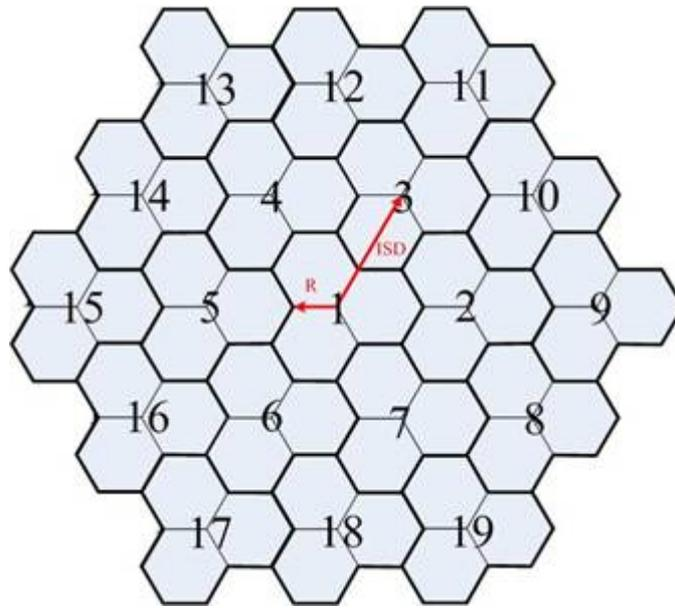
The cell layout of one LTE system is shifted over the other. Two base stations shifting of two operators are considered.
