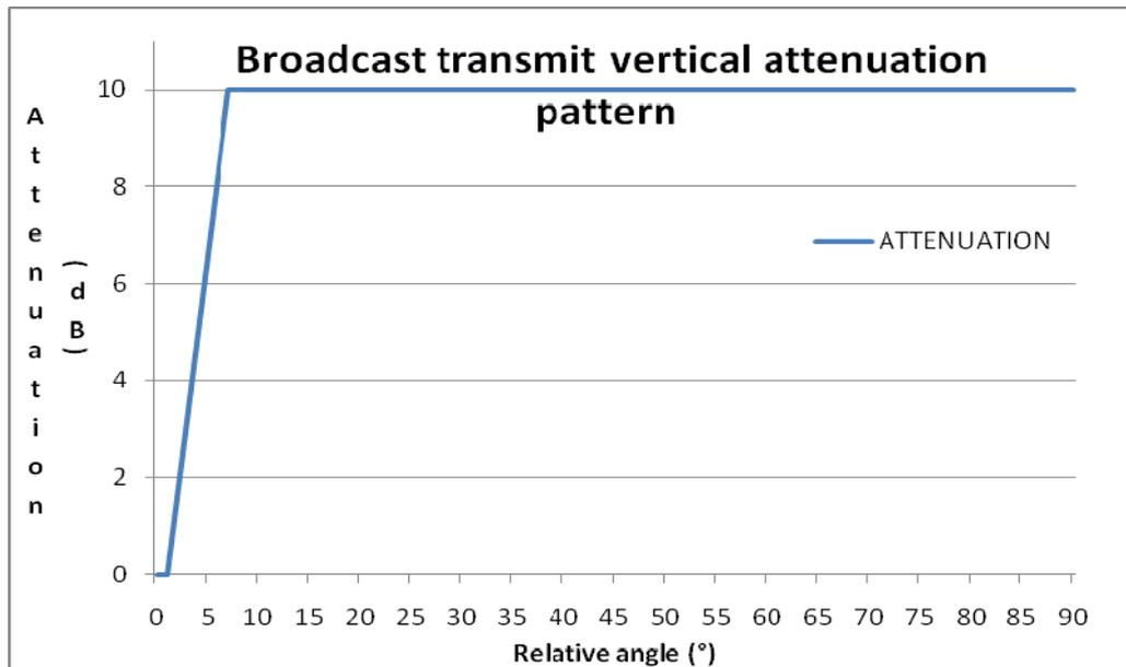
Broadcast transmitter antenna vertical pattern is given in Figure 2.4.3-1 with reference angle for broadcast transmission is 0°.
