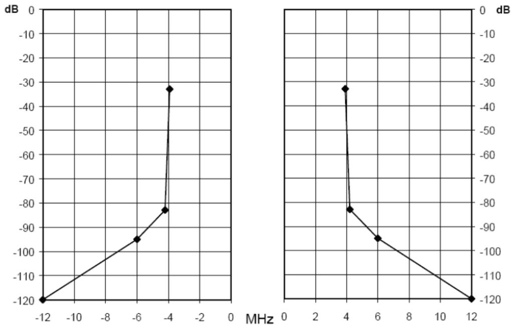
DTMB spectrum emission mask can be expressed by the following equation, where  $\Delta f$  corresponds to x-axis in the figure, and y corresponds to y-axis in the figure.
