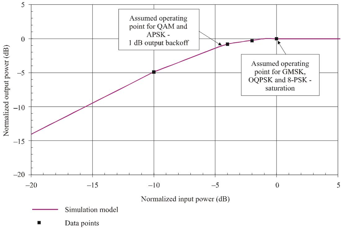
Note 1 – Because 8-PSK results collected with power amplifier operating in saturation, 8-PSK results can, at times, be worse than QAM.
