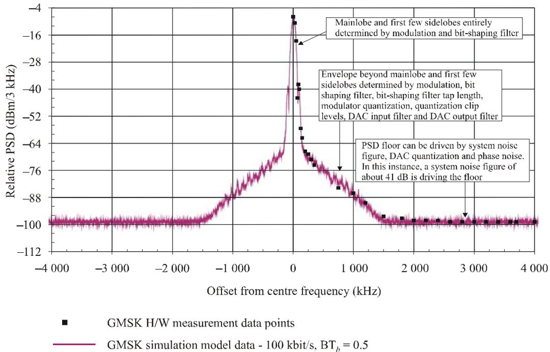
Note 1 – PSD generated based upon the low fidelity grade settings described in § 3.1 with the exception that 10-bit quantization with non-optimal clip levels was used. Additionally, no output diplexer was used.
