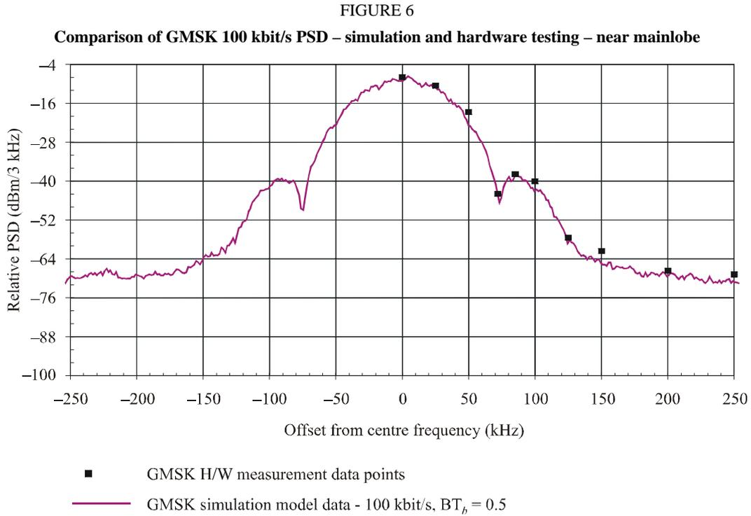
*Note 1* – PSD generated based upon the low fidelity grade settings described in § 3.1 with the exception that 10-bit quantization with non-optimal clip levels was used. Additionally, no output diplexer was used.
