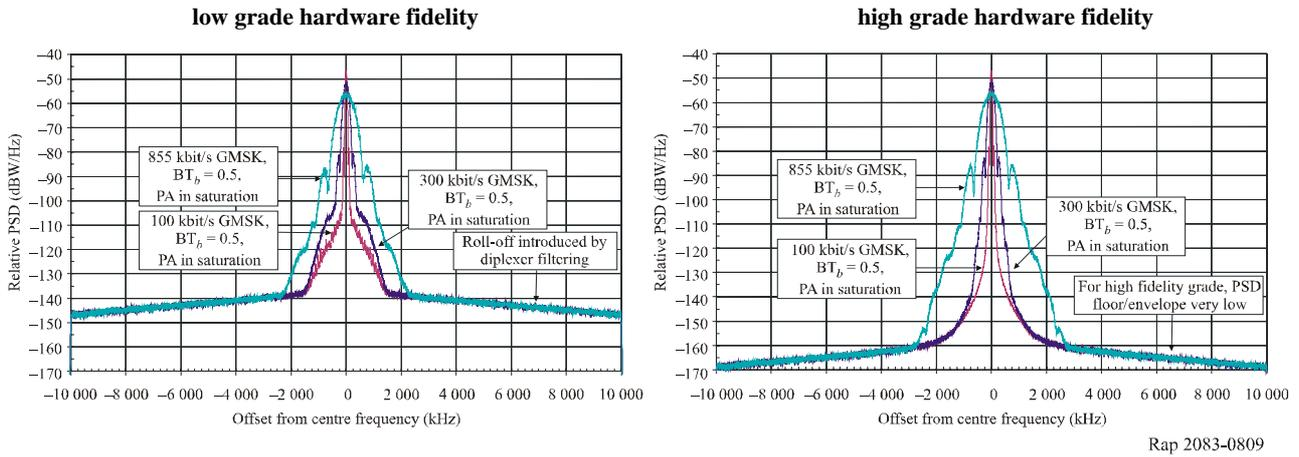
Figures 10 and 11 provide OQPSK/PM PSD data generated via simulation assuming, respectively, the hardware low- and high-fidelity grade settings.
