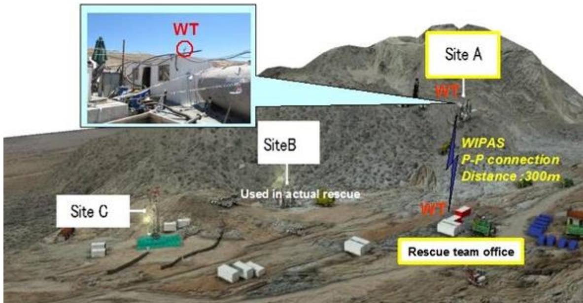
FIGURE 32 Example of a wireless link using WIPAS for emergency
