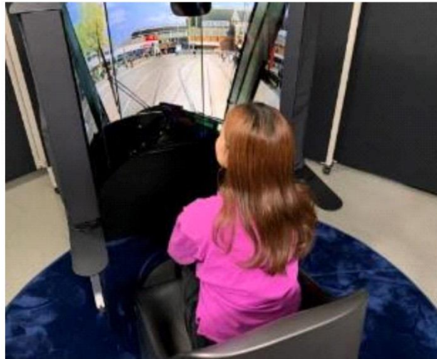
FIGURE 16 Immersive VR displays and haptic chair device
