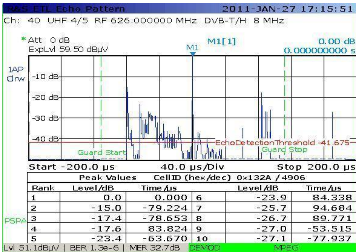
FIGURE 8 Impulse response for MUX4 at Dongo measurement point
