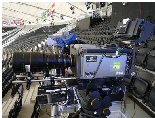
FIGURE 54 1.25-inch 4-CMOS camera and 5x lens
