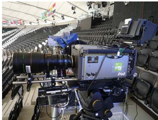
FIGURE 48 1.25-inch 4-CMOS camera and 5x lens
