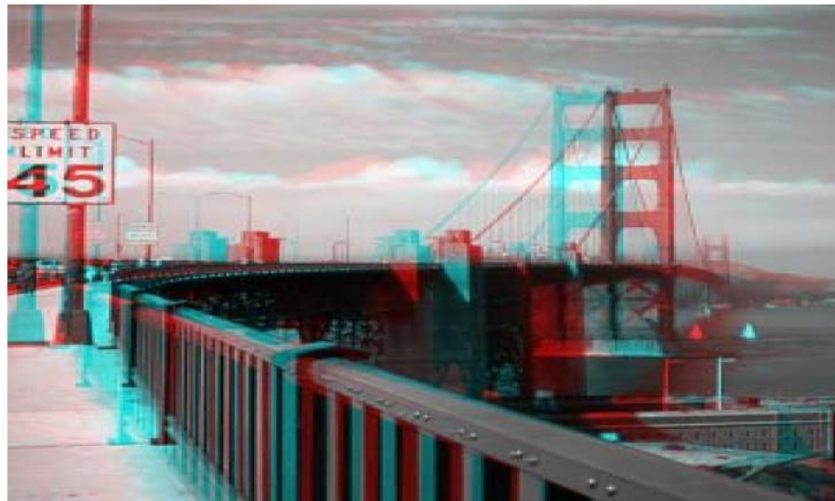
Figure 4: Red/Cyan anaglyph image as it is transmitted and appears on all TVs
