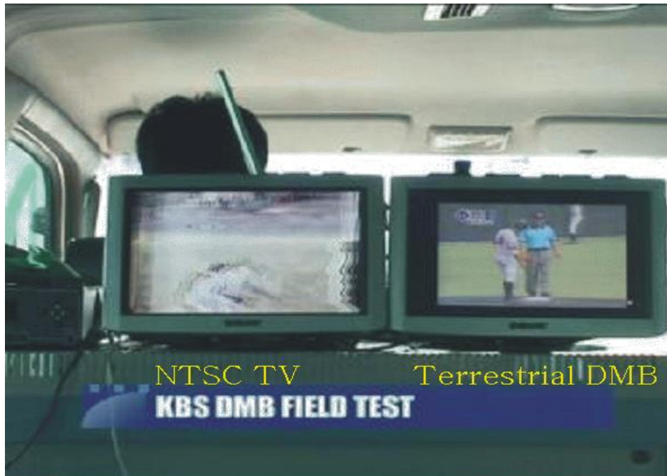
FIGURE 22 Reception comparison between NTSC and T-DMB
