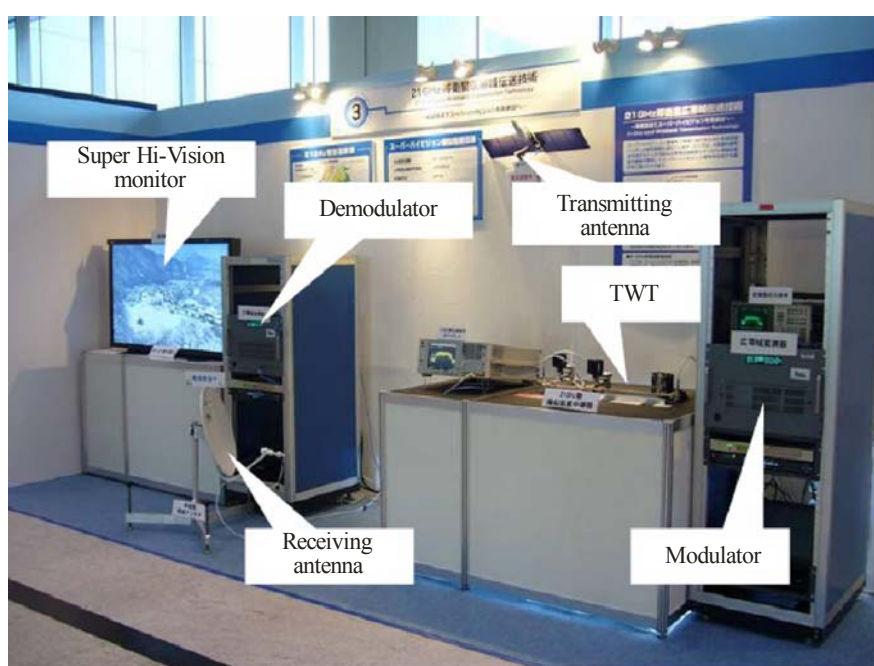
FIGURE 2 Transmission experiment in the 21 GHz-band
