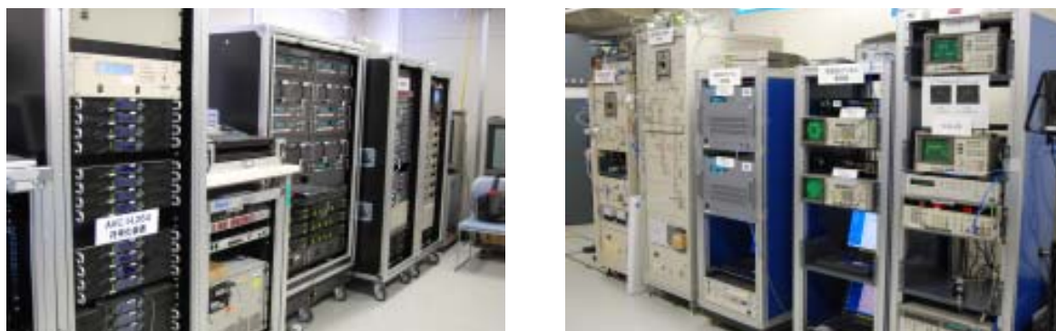
FIGURE 4 Indoor transmission experiment in the 21 GHz-band: Codec (left) and modem and transmission-path simulator (right)
