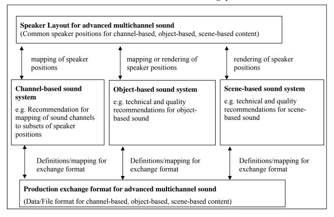
One important part of the framework specifies common speaker positions for advanced sound systems. This information can be independent of the approach of content representation and rendering. It is intended as a reference for describing advanced loudspeaker setups (e.g. in perceptual evaluations). For the definition of a possible speaker layout, it is necessary to gain a common base of knowledge about naming, positions and labelling of speakers in multichannel sound systems.
