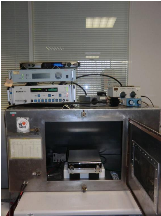
Wanted and interfering transmitters, clipper/Faraday Cage (at left) – measuring devices (At right)
