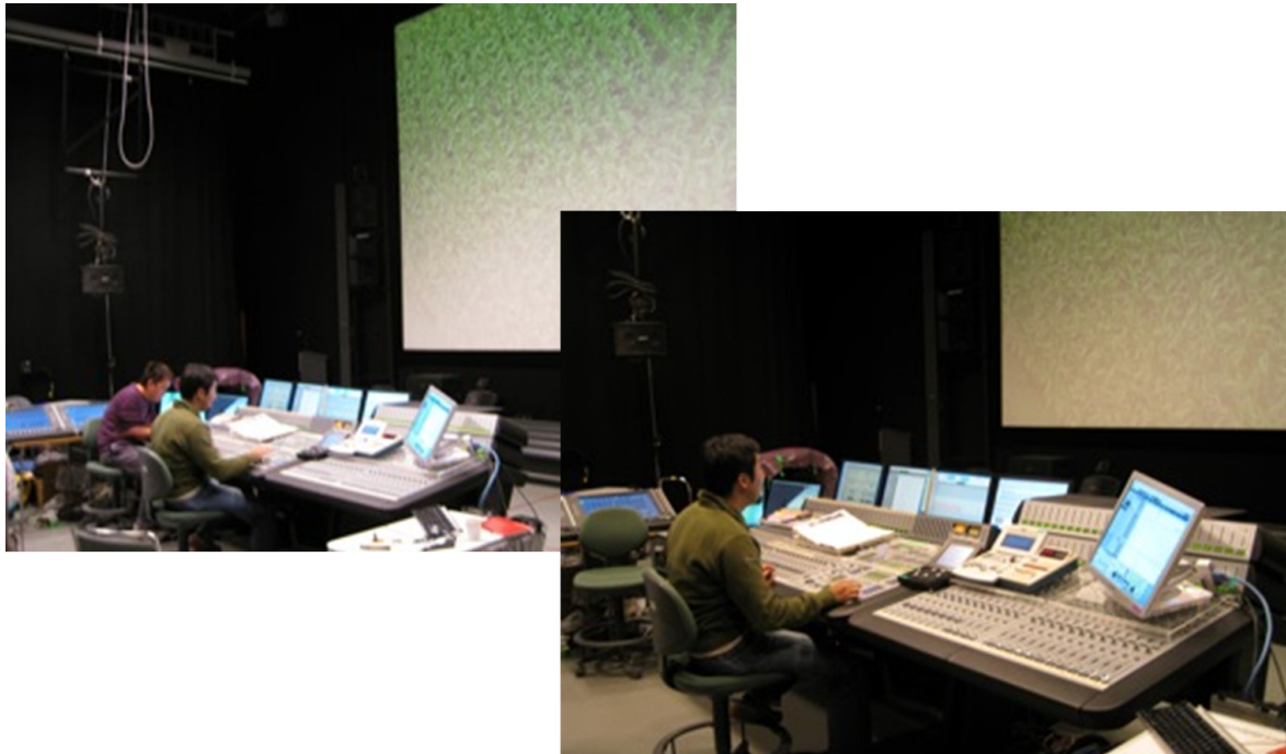
FIGURE 12 22.2 multichannel sound mixing console
