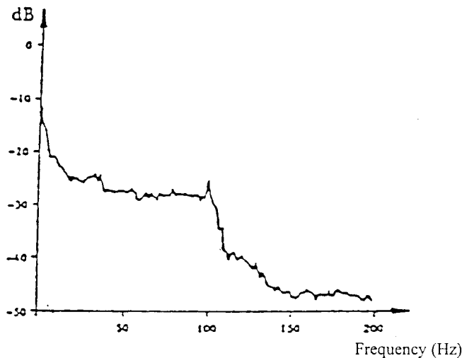
FIGURE 22 Spectrum of signal envelope (suburban area); vehicle speed: 40 km/h, frequency: 1.5 GHz [Jongejans, 1986]
