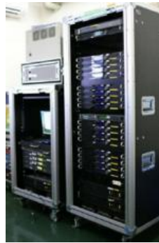
SHV encoder (Sapporo) and decoder (NHK STRL) (H.264, TS 100 Mbit/s)
