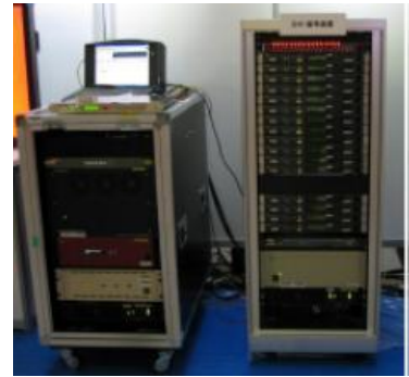
SHV encoder (Sapporo) and decoder (NHK STRL) (H.264, TS 100 Mbit/s)
