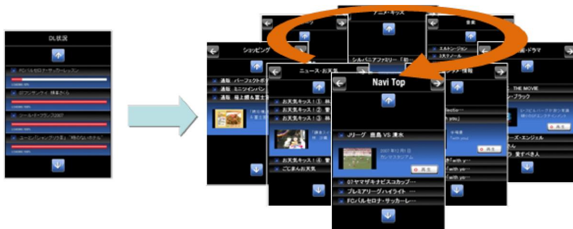
FIGURE 9.58 Example of filecasting service on a palmtop receiver
