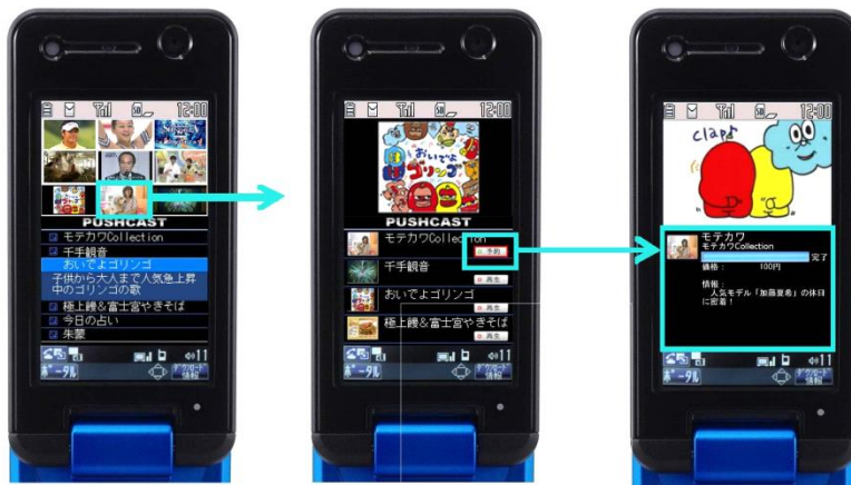
FIGURE 9.56 Example of filecasting
