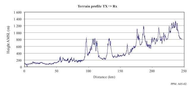
Interpolating on the 600 MHz and 2 000 MHz field strength tabulations (1% and 10% time) yields a predicted interfering signal of -4.07 dB( $\mu$ V/m) relative to 1 kW ERP. The receiver height correction and the terrain clearance angle correction are 23.41 dB and -12.68 dB, respectively. Finally, an adjustment of 30 dB is included to account for the transmitter power (1MW), which yields an interfering signal strength of 36.66 dB ( $\mu$ V/m).
