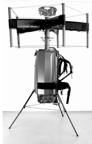
b) A 20-3 000 MHz antenna in deployed configuration where a compact receiver and DF is installed
