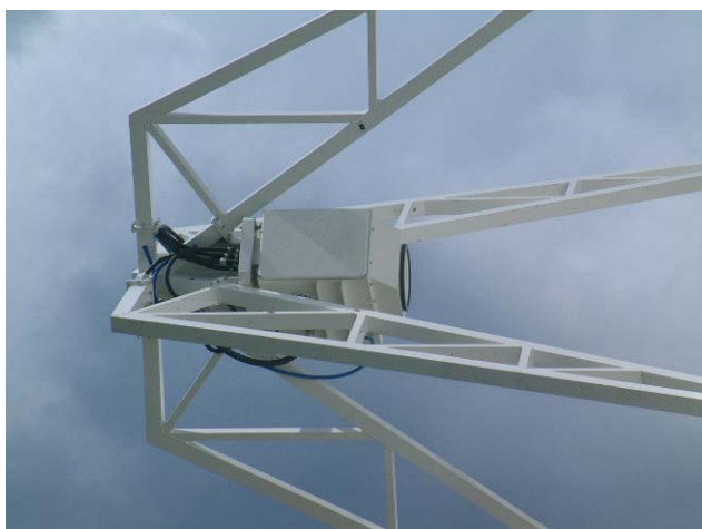
FIGURE 5.1-19 Multifeed mounted in prime focus
