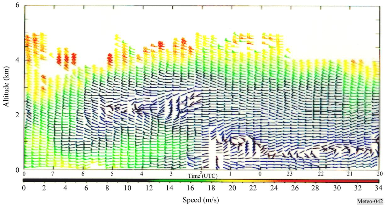
L-band WPRs (often called: boundary layer profilers) usually measure wind data at levels below a few kilometres. However, JMA WPRs collect data up to 5 km with the height resolution of 100-600 m, applying the pulse-compression technique, generating a high power transmission, and using a large-size antenna. All the WPRs are controlled from the PCC of the JMA headquarters in Tokyo. The main characteristics of the WPR are listed in Table 4-2.
