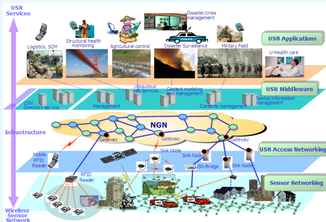
Figure 4-1: Schematic Layers of a Ubiquitous Sensor Network
