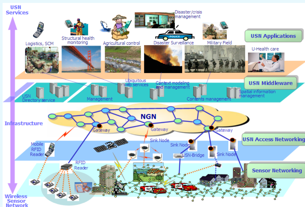
Figure 4-1: Schematic Layers of a Ubiquitous Sensor Network
