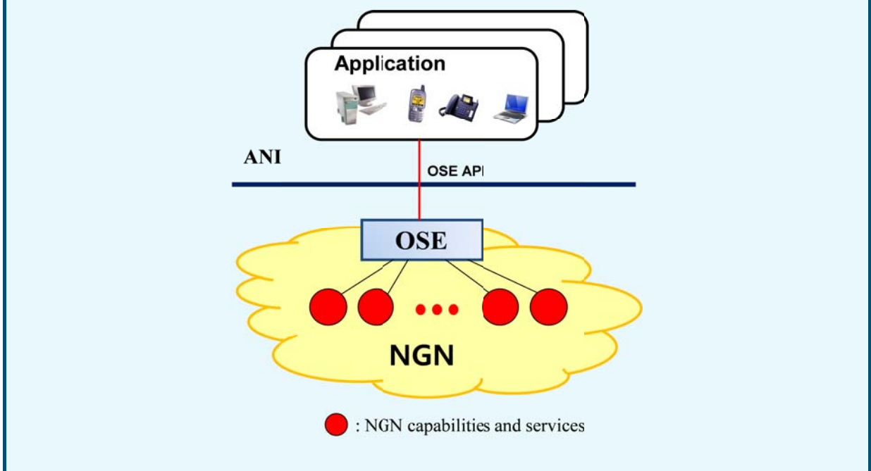
Figure 2-1: Open service environment capabilities in NGN
