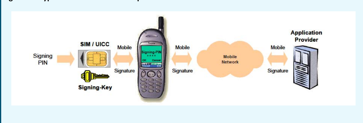
Figure 14: Typical mobile smartcard implementation
