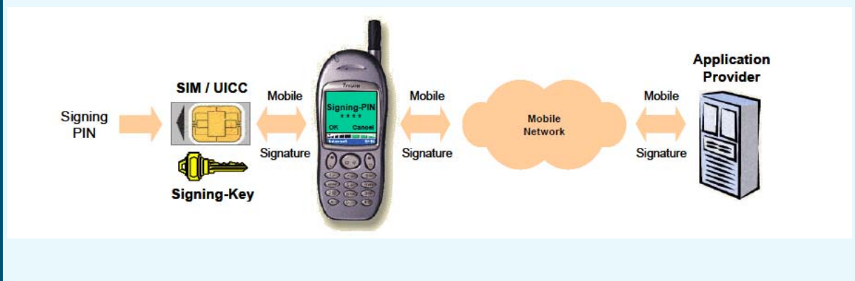
Figure 14: Typical mobile smartcard implementation
