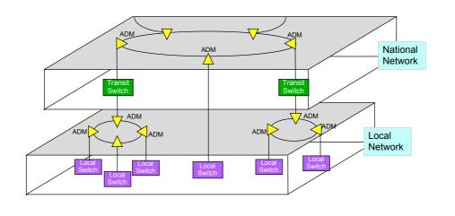
ALCALA supports two network design tasks, the first of which is configuration and topological design. Taking into account the switching configuration and existing outside plant constraints, it selects suitable mesh or multi-ring network structures.
