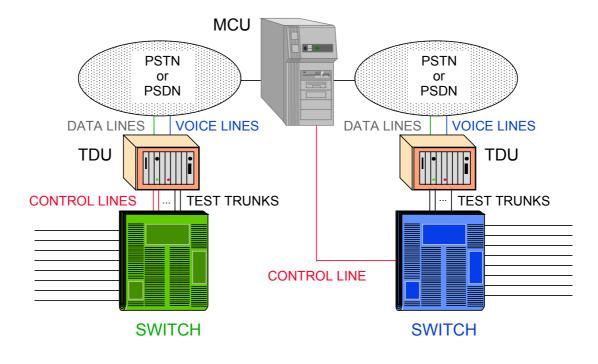
The MCU accesses the Switches either directly through the network, or through the TDU, depending on their Maintenance Facilities. For instance, all electro-mechanical Switches are accessed through TDU's.
