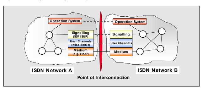
Figure 2.7.2 – Physical and logical linking of ISDN networks
