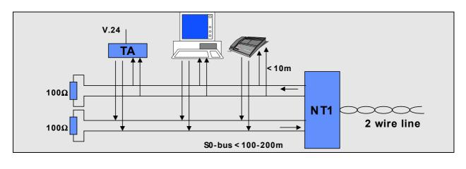
Up to eight ISDN Terminals (TE1) or ISDN Terminal Adapters (TA) can be connected to the  $S_0$ -Bus. Two of them can be used in parallel each accessing one of the B-channels. The terminals may be ISDN telephones, Group 4 Telefaxes or Data-Equipment like a PC with ISDN Adapter-Card. Additionally, terminals may also use the data packet service offered via the D-channel.
