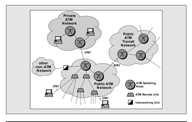
**Broadband ISDN inter-carrier interface (B-ICI)** – defines inter-switch communications in public networks (af-bici-0068.000).
