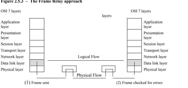
Figure 2.5.3 – The Frame Relay approach
