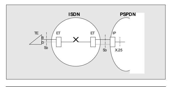
An ISDN terminal, TE, capable of X.25 Protocol or an X.25 DTE adapted to ISDN So-interface, is accessing the PSPDN via B-channel(s) terminating in an ISDN interworking Port unit, IP.
