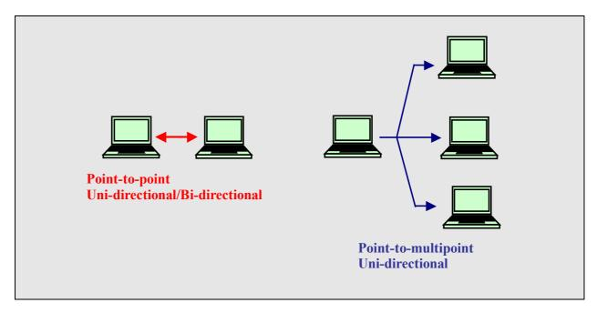
Point-to-multipoint connections are unidirectional, meaning that the root is allowed to transmit data to the leaves, and not leaves to the root or to each other.
