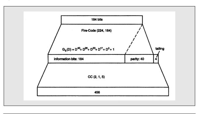
Figure 3.4 – FEC in SACCH, FACCH, BCCH, SDCCH, PCH and AGCH
