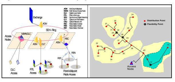
Figure A2 – Structure and one of the topologies of the access network
