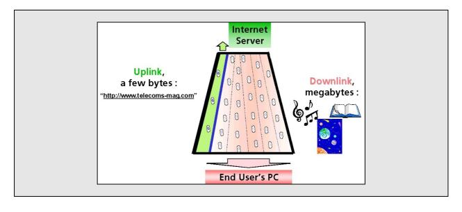
Thus the flow of information in user access to the Internet is commonly quite *asymmetric* in nature. Radio technologies that can dynamically adapt to asymmetry have a distinct advantage over those that do not. In particular, if the duplexing of two-way communications is achieved by means of time division duplex (TDD), it is significantly easier to adjust to asymmetry *in real time* than with frequency division duplex (FDD).
