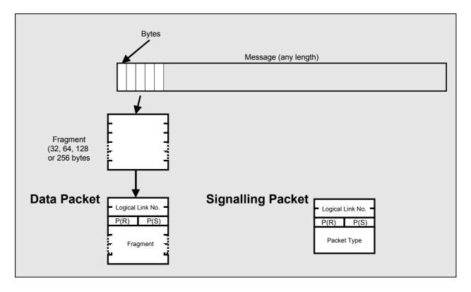
The frames are numbered modulo 8 (standard) or 128 (extended). Frames sent by one extremity of the link must be acknowledged by the other extremity. The procedure offers the possibility of anticipating the acknowledgements: each extremity can send a series of information frames (maximum 7 or 127 according to the case) without waiting for the acknowledgement of the first one. This device avoids dead time between frames and thus transmits at maximum speed.
