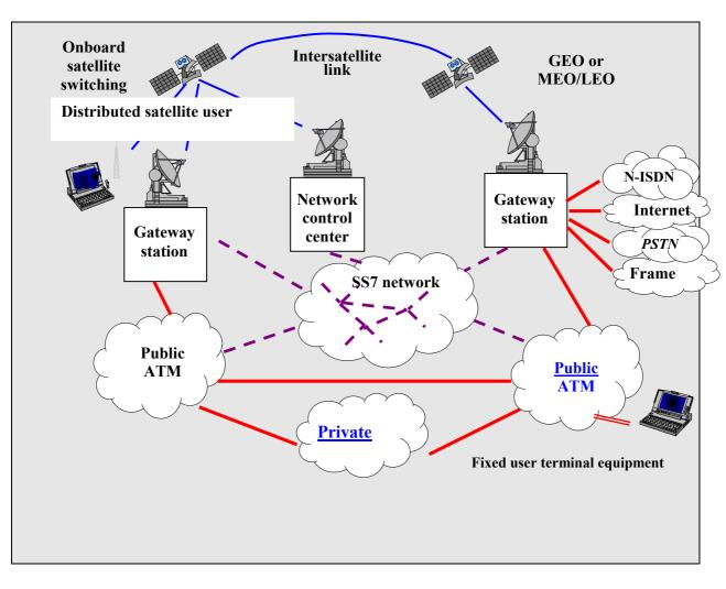
Figure 2.6.13 – Global ATM network, according to [3]-[4]
