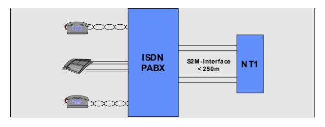
Due to the point-to-point characteristics of the interface no D-channel access mechanism is necessary. It is possible to con the 30 B-channels into bundles using only part of the 30 channels or to assign channels as incoming or outgoing channels only. 2.2.6 shows the channel structure at the  $S_{2M}$ -interface
