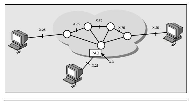
A DTE can be a terminal that does not implement the complete X.25 functionality. A DTE is connected to a DCE through a translation device called a packet assembler/disassembler (PAD). The operation of the terminal-to-PAD interface, the services offered by the PAD, and the interaction between the PAD and the host are defined by ITU-T Recommendations X.28, X.3, and X.29, respectively.
