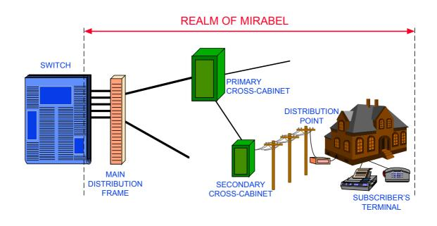
MIRABEL considers copper lines only, since the process is based on electrical tests. Any type of copper wires may be monitored. Even in the case of ISDN lines the wires are tested from an electrical point of view.
