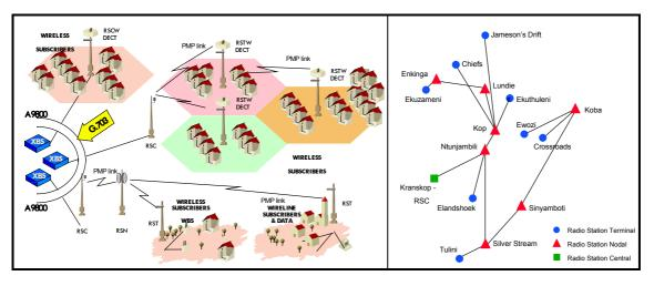
Alcatel is providing 288 000 lines of radio access equipment to the South African operator Telkom. The rural area of Kranskop (see Figure 6) has been selected as a pilot planning application with the objective of the exercise to locate and dimension the Alcatel 9800/DECT equipment. An exchange (Radio Station Central or RSC) serves the whole area via a point-to-multipoint microwave network.
