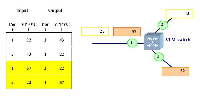
Figure 2.6.3 – ATM switch operation
