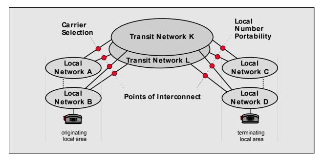
As indicated in the Figure 2.7.3, in case of a long distance call, carrier selection determines the call routing towards and interworking at the point of interconnection in the originating local area. In the terminating local call area, number portability requires new routing methods to select the point of interconnection to and appropriately inter-work with destination local networks.
