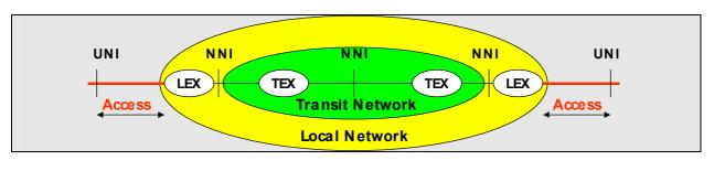
The ISDN reference configuration shown below structures the access as indicated in Figure 2.2.2 in functional blocks. Each of them is dedicated to a number of functions to be performed. Reference points separate the different functional blocks, Figure 2.2.3.
