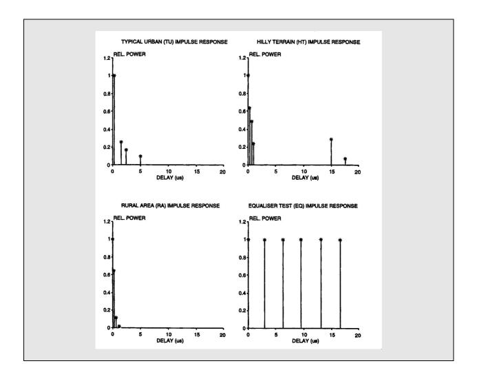
Figure 3.6 – Typical GSM channel impulse responses
