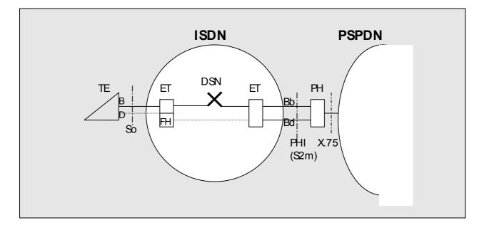
In the ETSI scenario the PH-function is located outside the ISDN, often close to the PSPDN, but still logically belonging to the ISDN. The PH is accessed via a standard Packet Handler Interface, PHI, which is physically an ISDN Primary Rate Interface.
