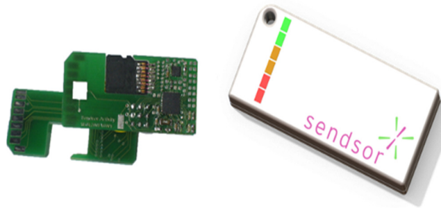
Figure 6: Miniaturized activity sensor for a vest pocket developed by Sendor GmbH
