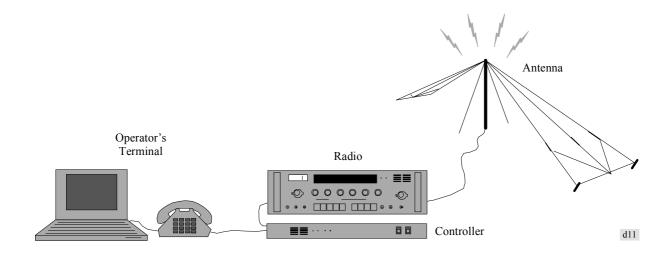
The main functions of the controller unit in an adaptive system are frequency management and link quality assessment, link preparation and establishment, link maintenance and disconnection.
