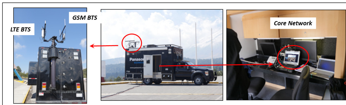
Figure 11A: Local Cellular System (LTE and GSM)
