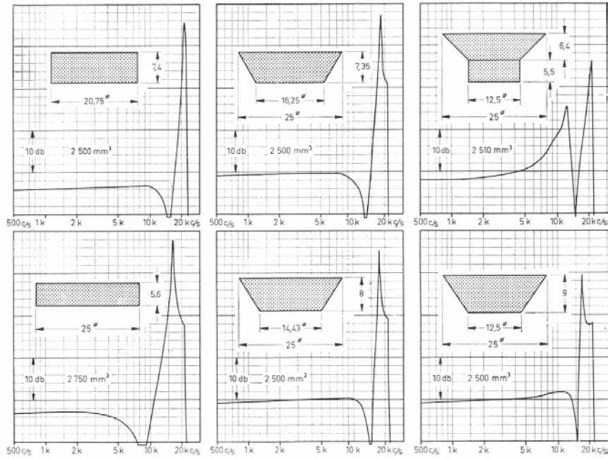
**Fig. 5** Frequency response obtained by a 1/2" condenser microphone receiver and transmitter mounted concentrically at the top and bottom of the variously shaped coupler volumes. Valid for the range 500-20000 Hz. All coupler dimensions are given in millimeters. Vertical scale 2dB per line, 50dB full scale.
