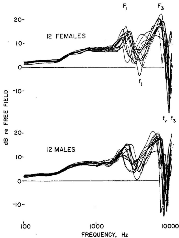
Fig. 13 Ear canal entrance sound pressures, 12 males, 12 females, sound source at 90° azimuth angle, 1m. Free field is the reference pressure condition.
