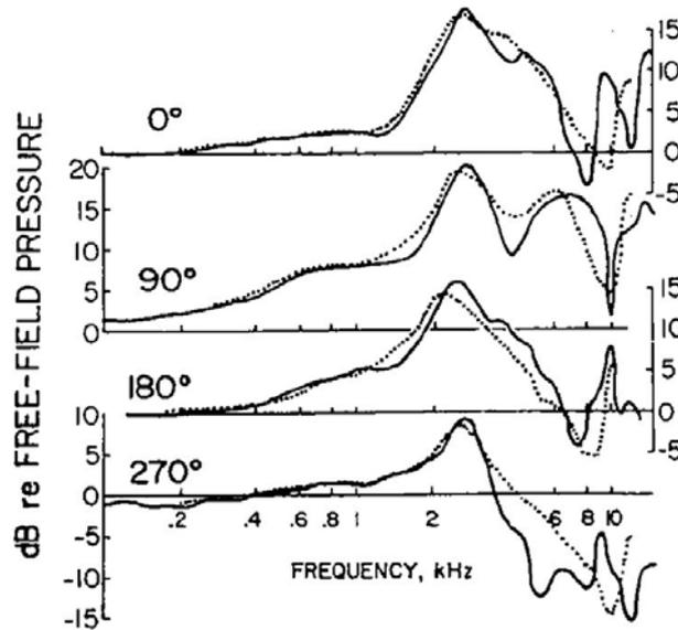
**Fig. 14 KEMAR Ear drum sound pressure for a free sound field with source azimuth angles of  $0^\circ$ ,  $90^\circ$ ,  $180^\circ$ , and  $270^\circ$ .**
