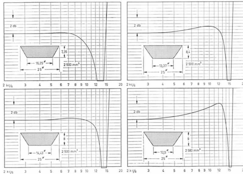
**Fig. 6** Detailed measurements to determine the optimum dimensions for the best possible linearity over the widest frequency range. 10dB full scale. 0.4 dB per line.
