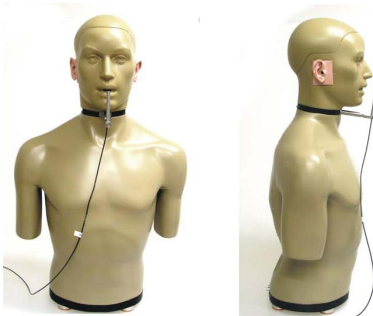
**Fig. 12 KEMAR with reference microphone for linearisation**
