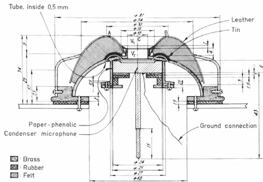
Fig. 1 Drawing of a French Artificial Ear as made by CNET
