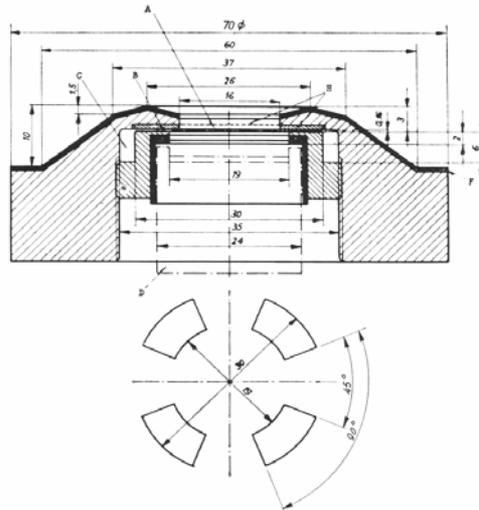
**Fig. 2 Drawing of a Swiss Artificial Ear as made by P.T.T.**
