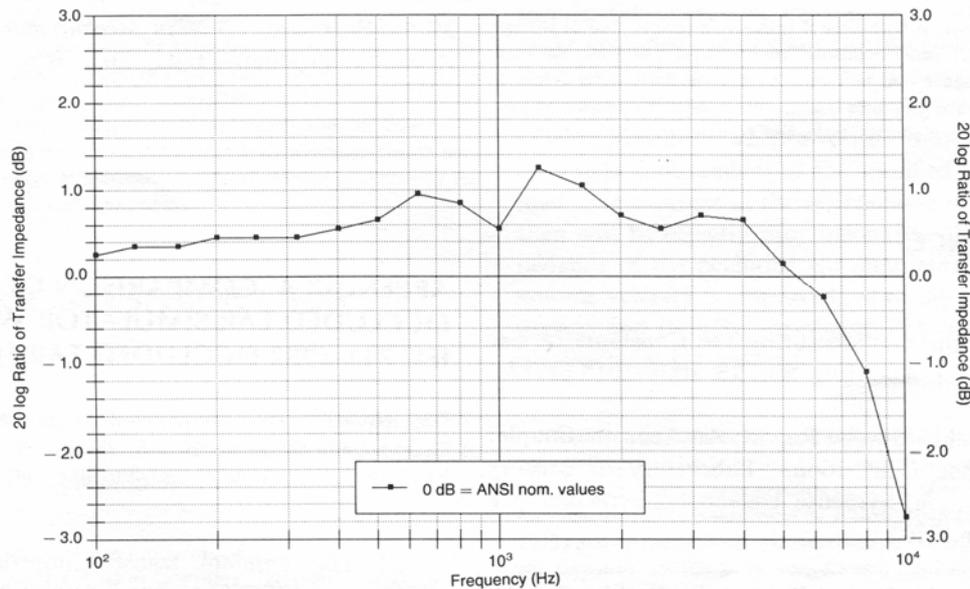
**Fig. 15 IEC Modulus values of the acoustic transfer impedance function from IEC 711-1982 relative to the ANSI modulus values of the acoustic transfer impedance function.**
