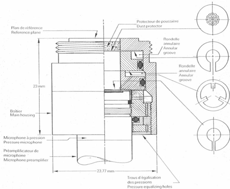
**Fig. 7 G.R.A.S. RA0045 occluded ear simulator as used in KEMAR**
