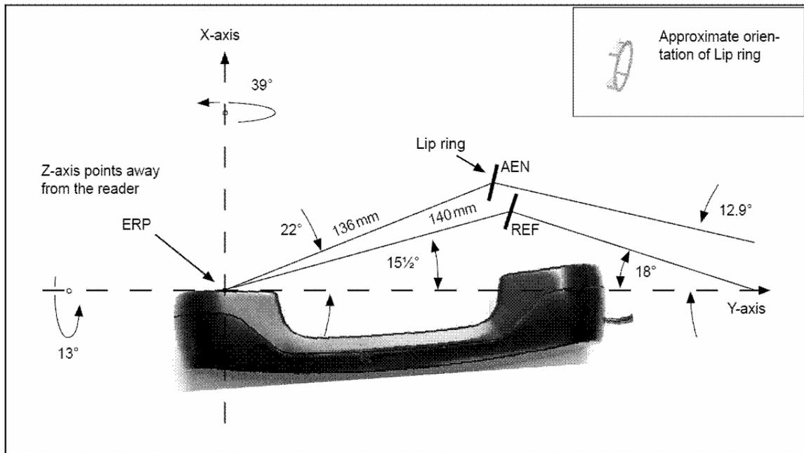
**Fig. 10c** Showing where the lip ring (of the type 44AA/44AB) should be for both AEN and REF positions. The angular distances of 39° and 13° (in that order) will move the handset from the AEN position to the LRGP.
