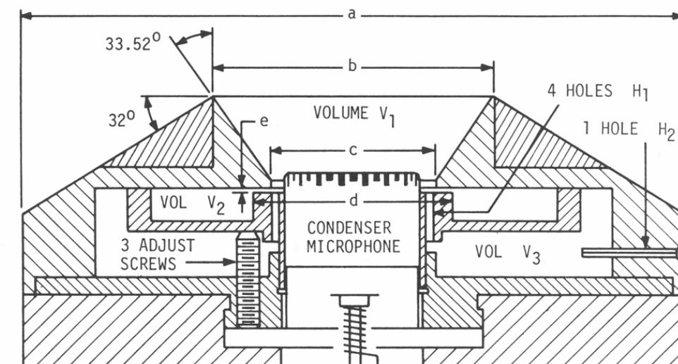
**Fig. 4 The IEC 60318-1 ear. The impedance and lumped parameter electrical network is shown in the IEC 60318-1 standard.**
