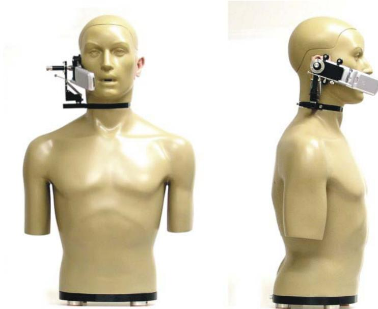
**Fig. 11 KEMAR with positioning device**
