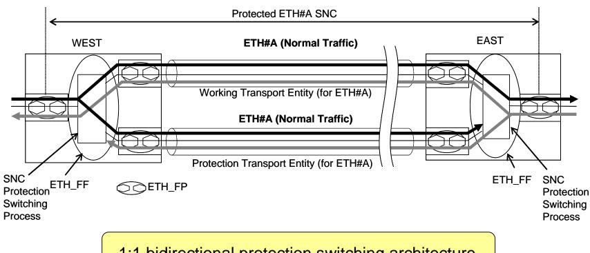
1:1 bidirectional protection switching architecture
