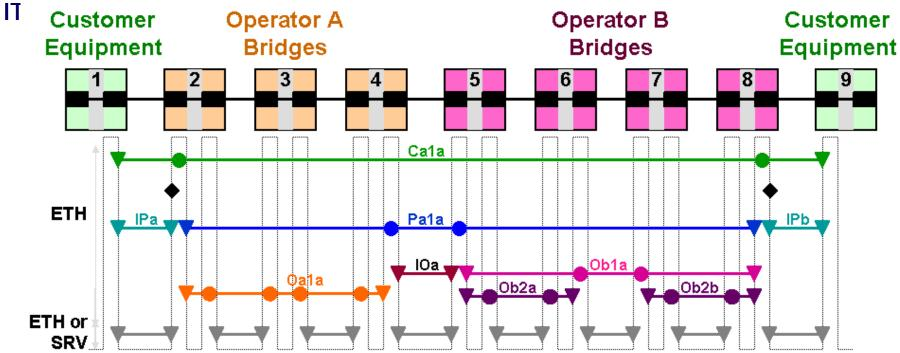
Multiple MEG levels are defined to allow running OAM in different spans
