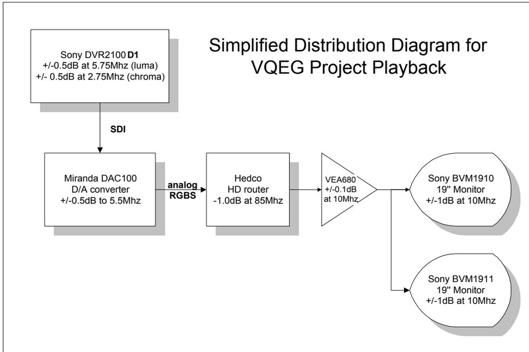
To characterize the video distribution system, a Tektronix TSG1001 test signal generator output was fed to the analog inputs of the Hedco router, using an 1125I/60 signal. A Tektronix 1780WFM was used to obtain measurements at the BVM-1911 input.
