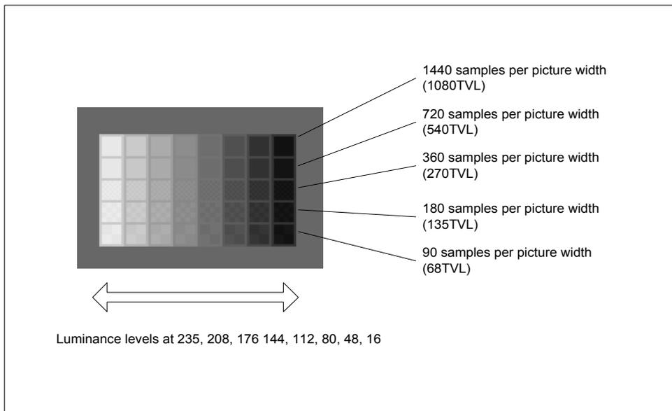
The subsections below show the estimated resolution in TVLs from visual inspection of the Briggs Pattern for each monitor used in the test.
