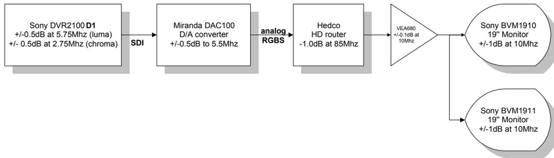
To characterize the video distribution system, a Tektronix TSG1001 test signal generator output was fed to the analog inputs of the Hedco router, using an 1125I/60 signal. A Tektronix 1780WFM was used to obtain measurements at the BVM-1911 input.
