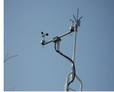
Wind Speed/Direction Sensor
