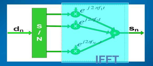
Orthogonal subcarriers  $\rightarrow$  high spectral efficiency FFT fast algorithm  $\rightarrow$  efficient implementation Low data rate on each subcarrier  $\rightarrow$  low ISI - Inter Symbol Interference Combing with advanced FEC - Forward Error Correction  $\rightarrow$  reducing burst errors
