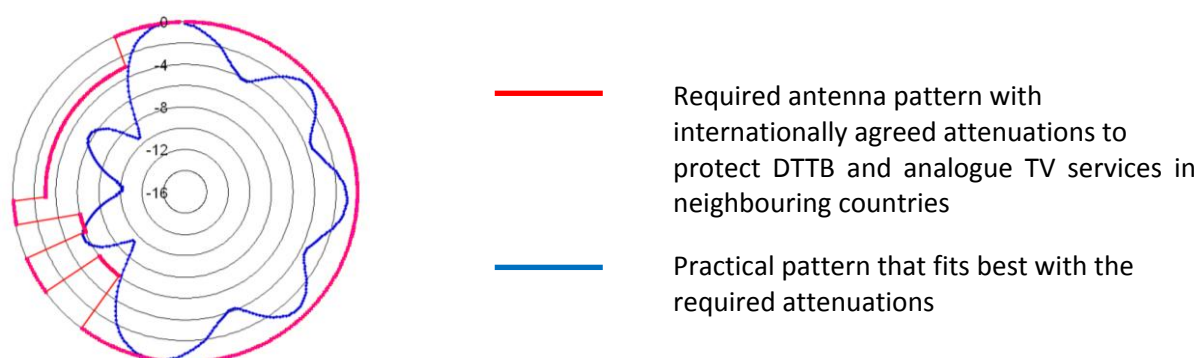
Figure 4.5.2: Example of a horizontal radiation pattern of a directional antenna
