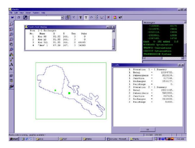
Optimization results – application of PLANITU for optimization of a local network with results for new exchange locations :
